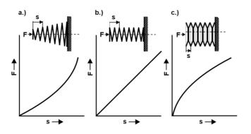
Figure 1.2: Spring characteristics a) progressive of a conical compression spring, b) linear of a cylindrical compression spring, c) degressive of a disc spring column
