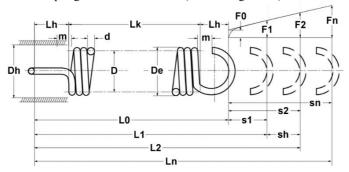
Figure 1.8: Theoretical Extension spring diagram
