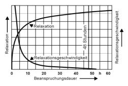
Figure 1.4: Time course of relaxation and relaxation speed for helical compression springs
