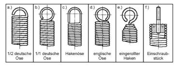
Figure 1.7: Common eye shapes: a.) half German eye; b.) whole German eye; c.) hook eye; d.) English eye; e.) rolled-in hook; f.) screw-in piece
