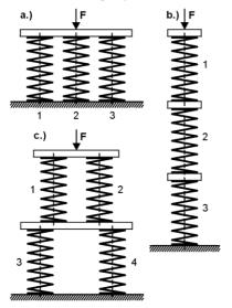
Figure 1.5: Spring systems; a) parallel connection; b) series connection; c) mixed connection
