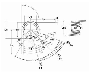
Figure 1.9: Theoretical torsion spring diagram
