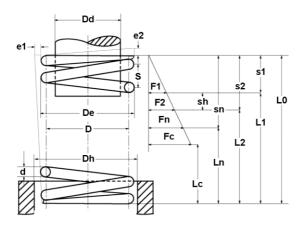
Figure 1.6: Theoretical compression spring diagram
